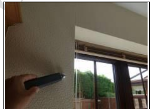
Testing for lateral dampness
