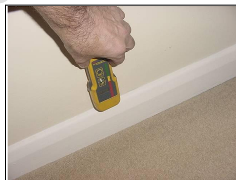
Testing for and finding minor rising damp
