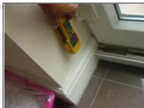
Checking for Rising Damp
