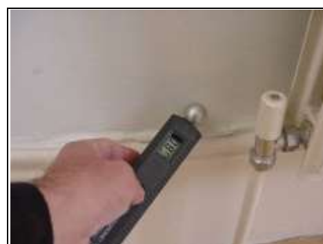
High damp meter reading
