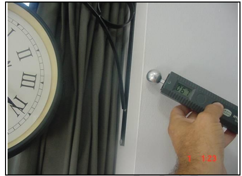
Testing for lateral dampness
