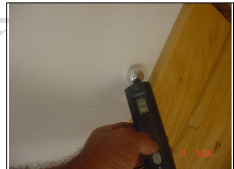
Testing for rising damp
