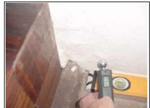
High readings near where staircase has been removed
