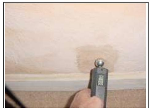
Ground floor testing area of plaster that has come away in hallway-
