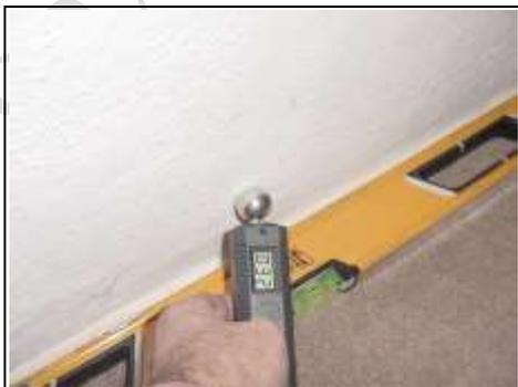
Taking readings above where the sole plate would be
