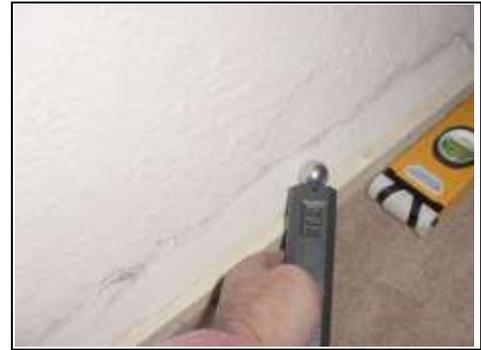
Damp readings taken where the sole plate should be are slightly high
